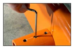
If the Shield Plate (1) is tight against the face of the wheel then no further adjustment is required. If, however, there is a gap between the back face of the Shield Plate (1) and the face of the wheel then Spacer Rings (5) must be used.
