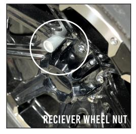
Once you have removed one of the wheel nuts, the Receiver Wheel Nut (4) can be fitted using the Wheel Wrench Adapter (10) which enables you to use a standard 19mm wheel wrench (see Fig.B). The Receiver Wheel Nut (4) should be tightened to the correct torque setting for your wheels.
