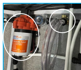
PUMP & 3-WAY VALVE FIGURE C
