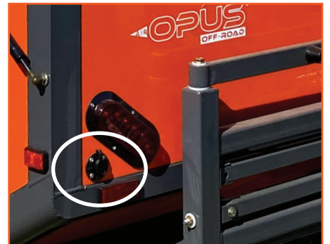
SOLAR PANEL PORT
