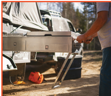
Slide open your kitchen & fridge. Connect your quick connects and fold down your kitchen support leg. Set up your sink drain and waste water carrier
