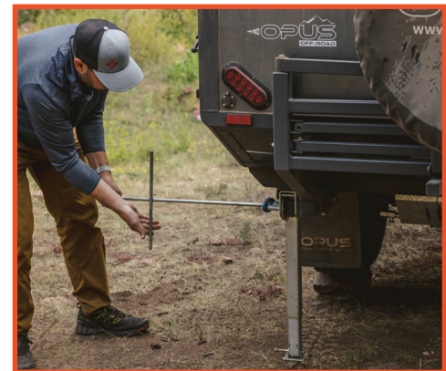
Whilst the tent is inflating, fold down your corner steadies & stabilize your trailer.
