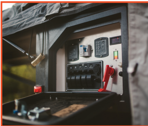
Turn on compressor: Ensure all 5 quick release valves on the driver's side are closed.
