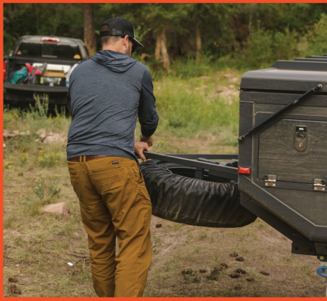
Lower the tongue jack. Release the spare wheel carrier to the horizontal position
