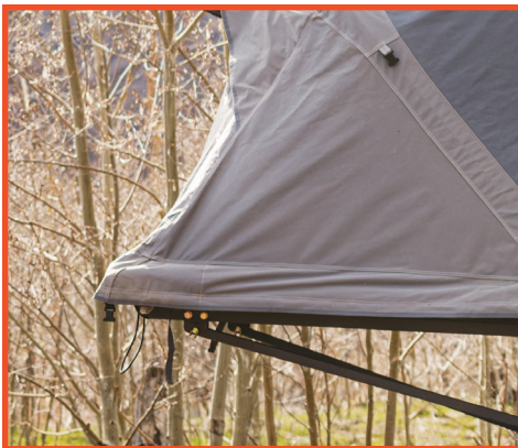
Pull the tent over the bed end corners & fix the bed support arms in place
