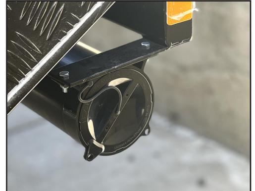
Located on each potable water tank you will find a draining valve at the lowest point of the tank. When packing away the OP15 complete the following process to drain the system of any excess water.
