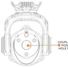
COUPLING UNLOCKED POSITION, TOW PIN HOLE MUST BE CLEAR
