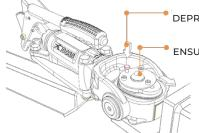
DEPRESS RED BUTTON FOR SPRING LOADED SLIDE TO LOCK COUPLING TO VEHICLE
